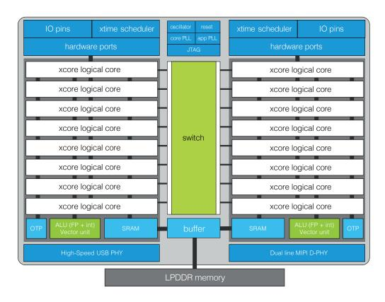
The xcore architecture is scalable. A standard device like xcore.ai contains two tiles (1 MByte of memory, up to 38.4 GMACC/s), two such devices can be put side by side on a PCB and programmed as a single system, providing 2 MByte of memory with up to 76.8 GMACC/s. This
