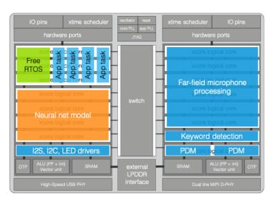
The flexible support of all classes of compute means that fully integrated system solutions can be supported on xcore, which drive maximum economy on the bill of materials.
