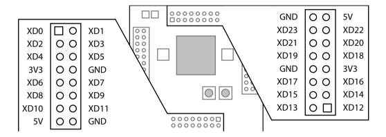
Each expansion header provides a bank of 12 I/O pins, which are mapped to the ports as described in the table on the next page, and four power/ground pins.
