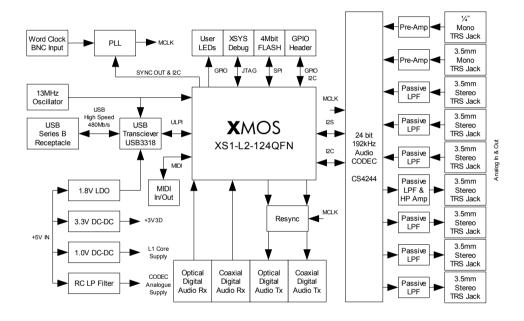
The XS1-L2 event-driven processor communicates with the USB host via a ULPI USB transceiver at the 480Mb/s high-speed rate. The XS1-L2 controls the streaming of audio data over the USB connection and direct I<sup>2</sup>S interface to the audio CODEC, digital streams and MIDI communications. Multiple additional functions (e.g. Mixers/DSP etc.) can be implemented by modifications to the standard software.
