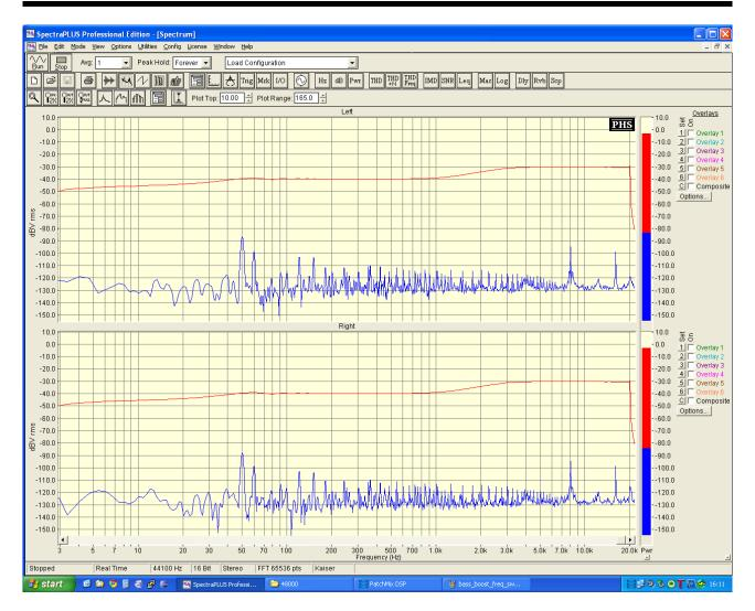
Figure 4: Frequency response for bass boost EQ setting
