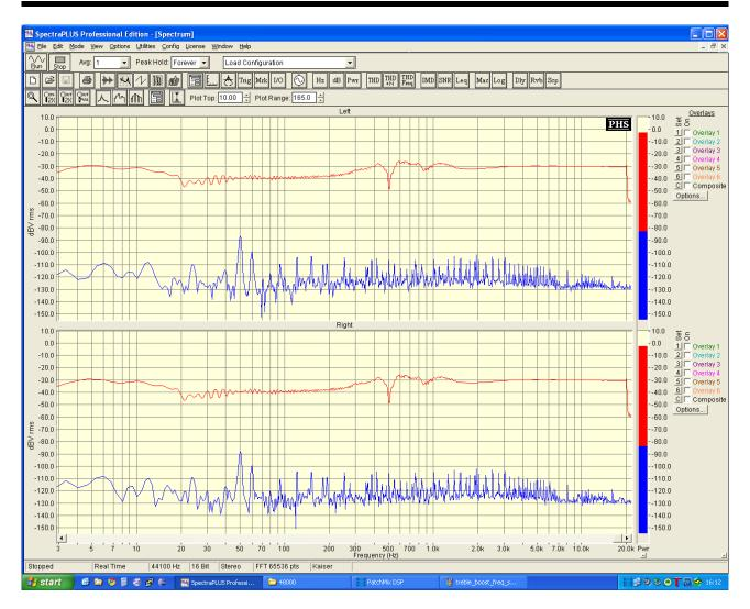
Figure 5: Frequency response for all filters
