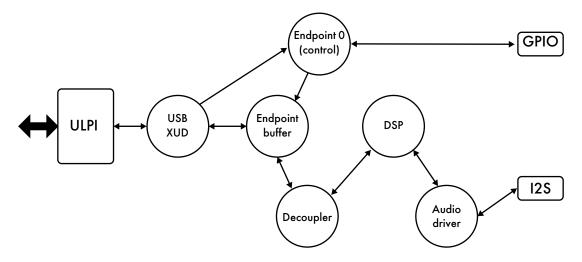
Figure 1: L1 USB Audio software core diagram with DSP core
