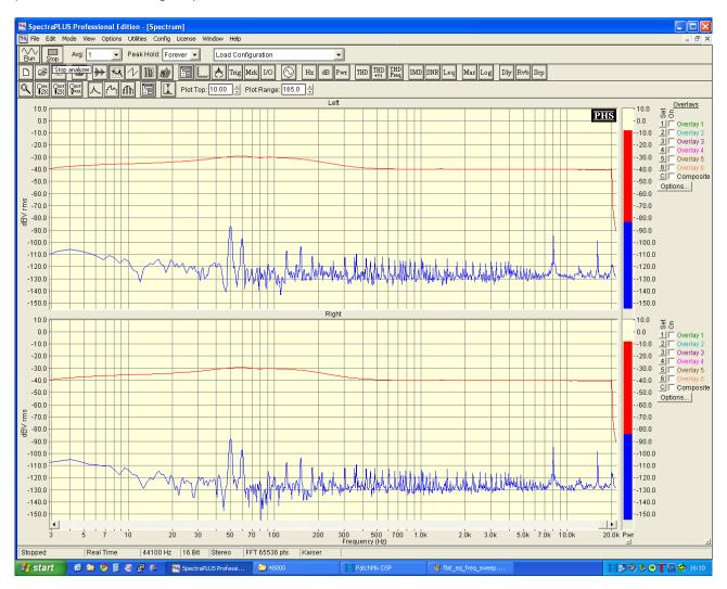
Figure 3: Frequency response for bass boost EQ setting
