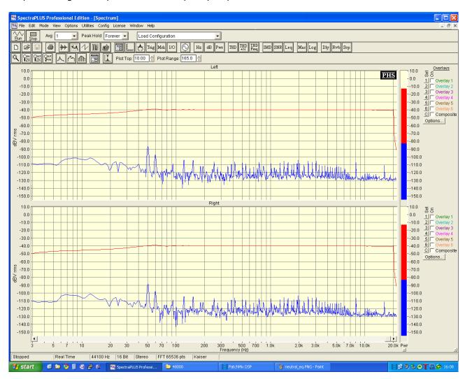
Figure 2: Frequency response for neutral EQ setting
