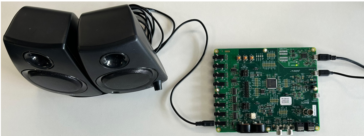
Fig. 2.1: XK-AUDIO-316-MC-AB with both USB cables connected and a pair of speakers connect to OUT 1/2
