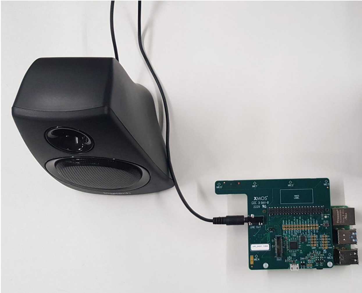
Fig. 2.4: XVF3800 demo example layout
