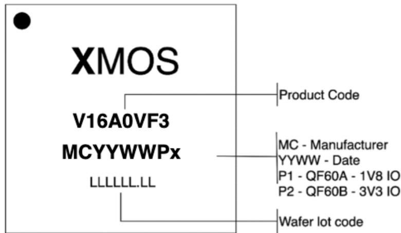
Fig. 8.2: XVF3800 Package Marking
