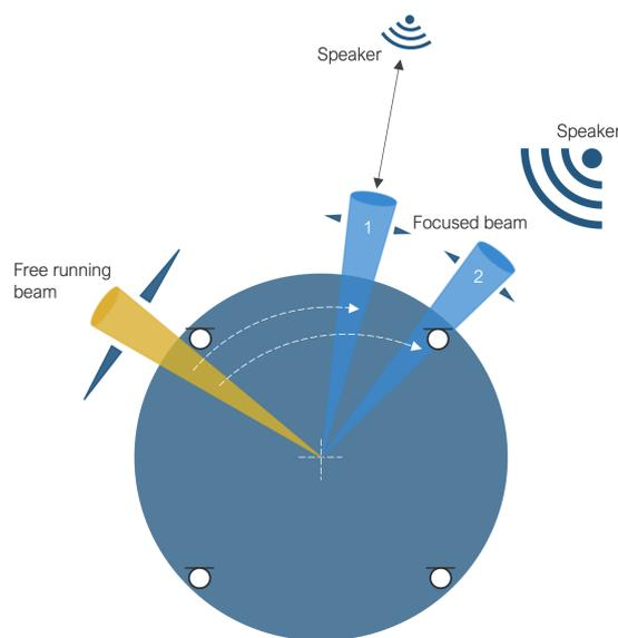
Fig. 3.2: Beamformer Operation
